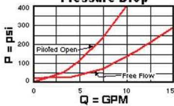
Free Flow and Piloted Open Pressure Drop
