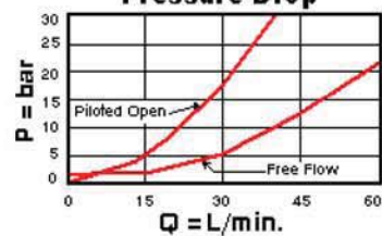
Free Flow and Piloted Open Pressure Drop
